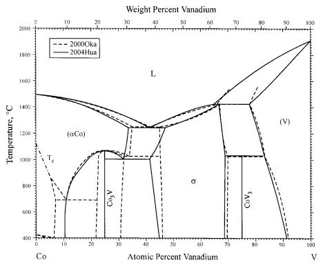
**Fig. 1** Co-V phase diagram
